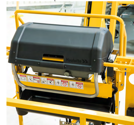
Control box protected by high-strength composite housing
