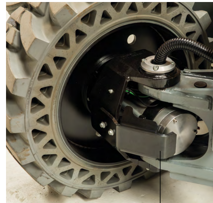
Thick protection shields around traction motors
