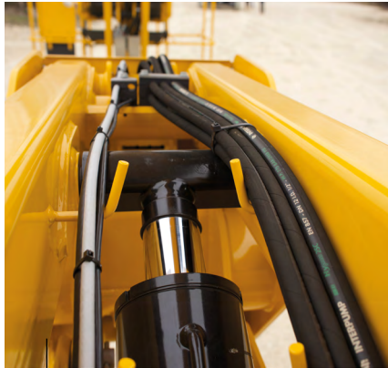
Guide bushings for cables and hoses
