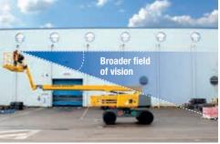
Due to the size of the boom, users may lack visibility when driving, potentially causing accidents.
