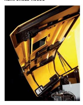
To withstand the test of time, impacts and damage during transport, cover hoods feature a metallic framework for extreme rigidity and sturdiness.
