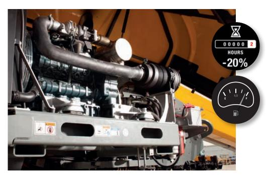
When operators are working at height, the engine often runs for no reason, resulting in the hourmeter counting hours unnecessarily. That is why the HT28 range is equipped with the innovative STOP Emission System that automatically stops and restarts the engine.
