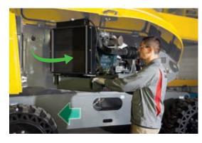
The HT28 range is equipped with a swing-out engine tray for direct access to key components.
