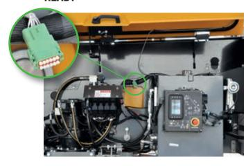
For fleet management the HT28 range is equipped with a universal telematics connector as standard.
