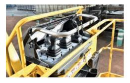
The HT28 range is equipped with a secondary guarding system: the HAULOTTE ACTIV'Shield<sup>©</sup> Bar 2.0 (standard or optional depending on models).
